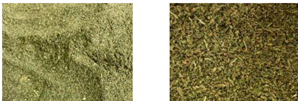
Fig. 3: Cannabis after grinding in the SM 300 foodGrade, left: using a 4 mm bottom sieve and grinding at 3000 rpm, right, using a 10 mm bottom sieve and grinding at 700 rpm
