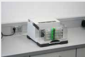
Fig. 5: Mixer Mill MM 400 with adapter for 8 conical centrifuge tubes
