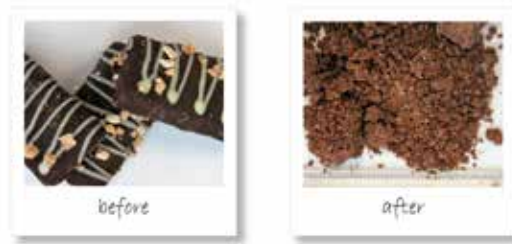
Fig. 11: Cookies before (left) and after pulverization in the Knife Mill GM 200 (right)
