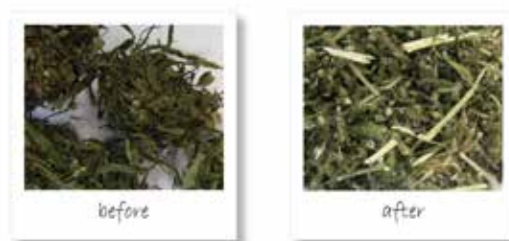
Fig. 2: Initial hemp sample (left) and after size reduction in the SM 400 XL (right)
