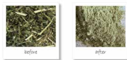
Fig. 4: After pre-cutting in the SM 400 (left) the sample is pulverized to <0.5 mm in the ZM 200
