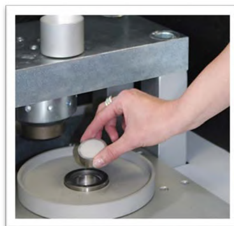
Fig. 3: Smooth and stable pellet produced in a Pellet Press PP 40
