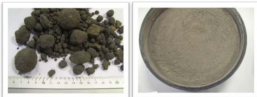
Fig. 2: Cement clinker sample before (left) and after (right) grinding in the RS 300 XL.
