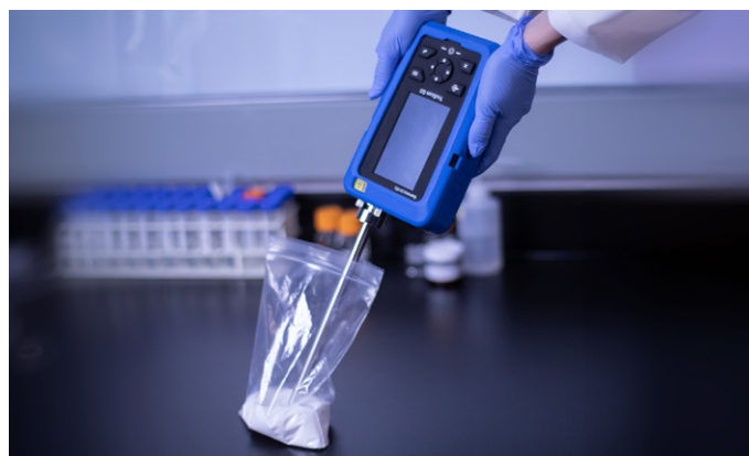
The TruScan G3, powered by Raman spectroscopy, provides field-ready solutions in support of the war on pharmaceutical counterfeiters.
