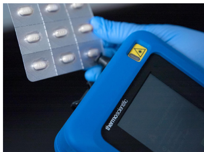
The TruScan G3 analyzer can be used in the field to provide rapid identification of counterfeit pharmaceuticals.
