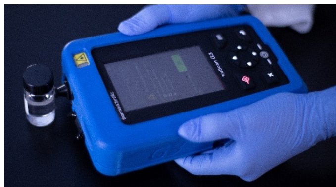
Figure 1. TruScan G3 handheld material identity verification system based on Raman spectroscopic technology - shown with accessories in top image.
